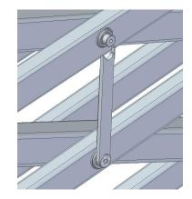
3 Lower the platform until the safety arm rests securely on the shaft. Keep clear of the safety arm when lowering the platform.
