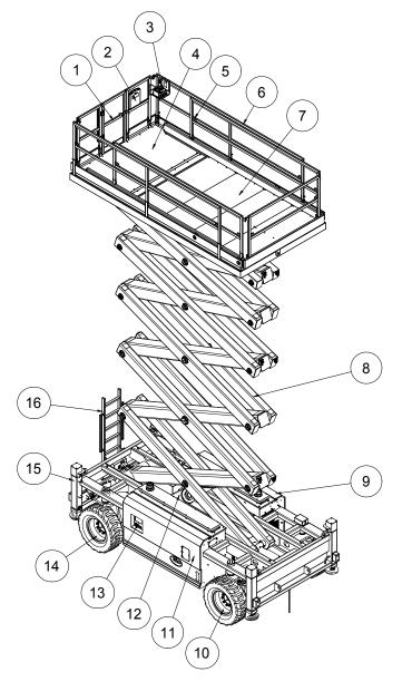
1 Platform entry gate 9 Engine(behind cover) 2 Manual storage containers 10 Rear wheel 3 Platform controls 11 Hydraulic tanks . Fuel tanks (behind cover) 4 Main Platform 12 Lift Cylinder 5 Lanyard anchorage point 13 Ground controls 6 Platform guard rails 14 Front wheel 7 Platform extensions 15 Outrigger 8 Scissor Arms 16.Entry ladder
