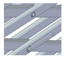
2 Remove the screw and rotate upward to a vertical position
